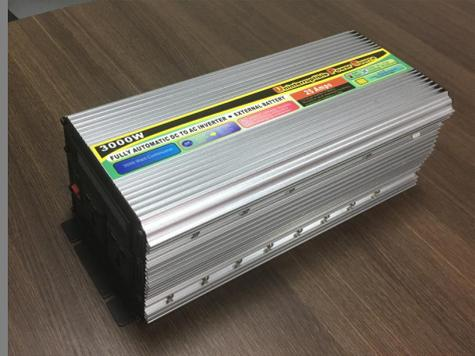
This power inverter convert DC 12V or DC 24V of the storage batteries into AC 110V or AC 220V, and also charge the storage batteries by converting the AC to DC when there is AC power supply. Briefly to say, when AC unavailabe, it convert DC to AC, when AC available, it supply AC output directly and charge the storage batteries.
